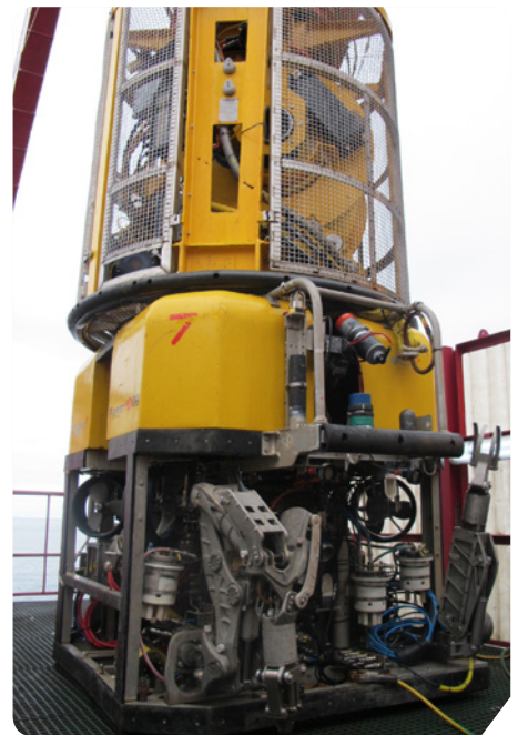
Workclass ROVs allows underwater inspection from vessels.
