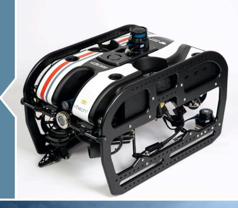
The vLBV® represents an evolution in small, capable, vectored MiniROV systems. Four powerful 100 mm (4") horizontal thrusters, arranged in a vectored format, offer nearly equal horizontal thrust in all 360-degrees of flight. The horizontal thrusters can be manually adjusted to bias thrust in the forward direction for extreme pulling power. This works well in applications such as long internal pipe penetrations and high forward currents.
